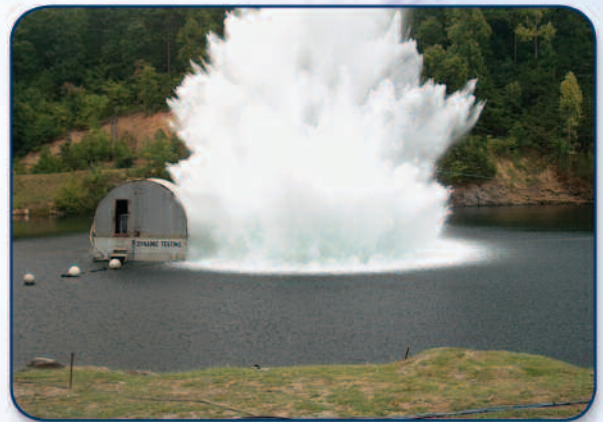
NTS' full spectrum test and research facilities are capable of managing your environmental test requirements, including MIL-S-901 high impact, heavyweight shock testing.
