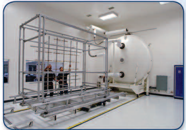
Special test environments are required to simulate space conditions in order to evaluate the life expectancy of today's communications and military satellites.
