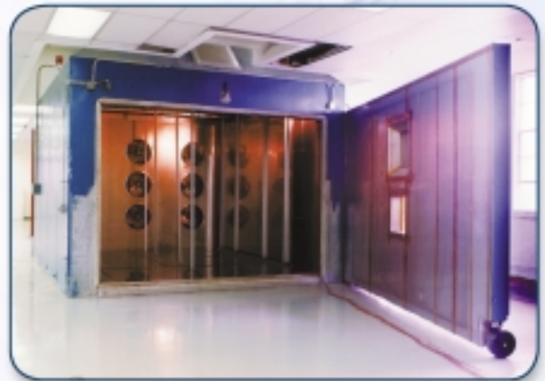
Thermal cycling and aging tests at 125° C/ minute transition rates are conducted in controlled-environment chambers. Photogrammetry and low oxygen test capabilities are available.
