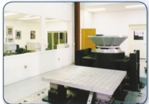
Transportation, aircraft and spacecraft vibration and shock conditions can be simulated and combined with environmental parameters such as thermal shock to validate product reliability.
