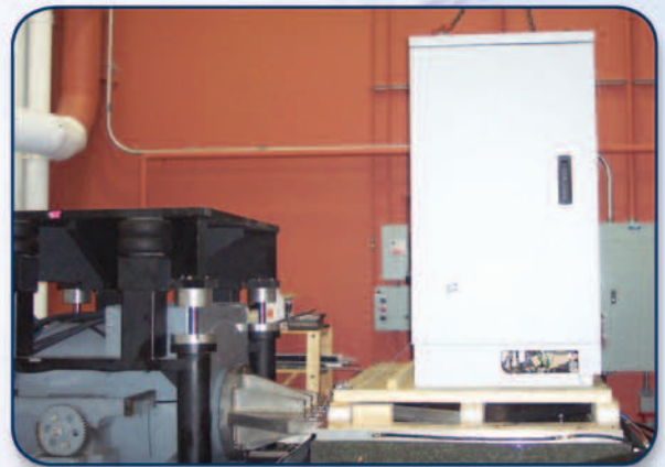
Vibration testing for up to 2500lbs payload.
