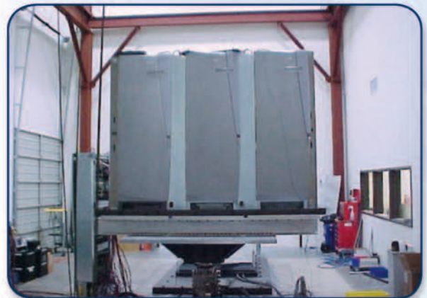
Seismic Test, Three Bays Rack, up to 3500lbs (Earthquake test)
