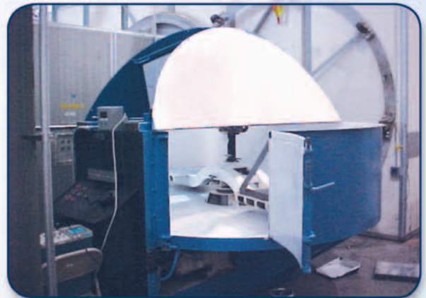
Centrifuge, 34" Armlength, up to 400rpm
