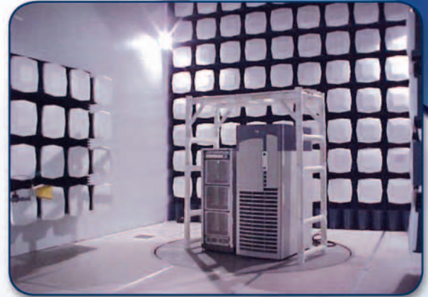
EMI/EMC Test in 3 Meter Semi Anechoic Chamber (FCC Certified Chamber)
