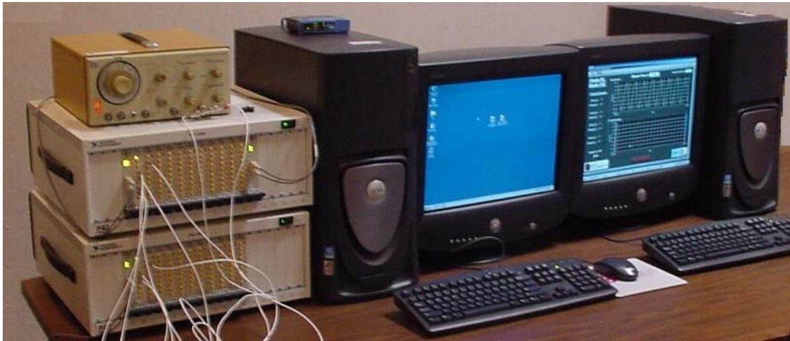
Figure 2. VTS Hardware Setup for a Two Workstation, Two PXI Test Configuration
